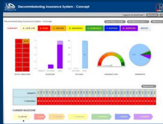
The IDEAS Activity screen is at the core of the system, allowing users to manage the entire decommissioning process using a clear and logical interface.
